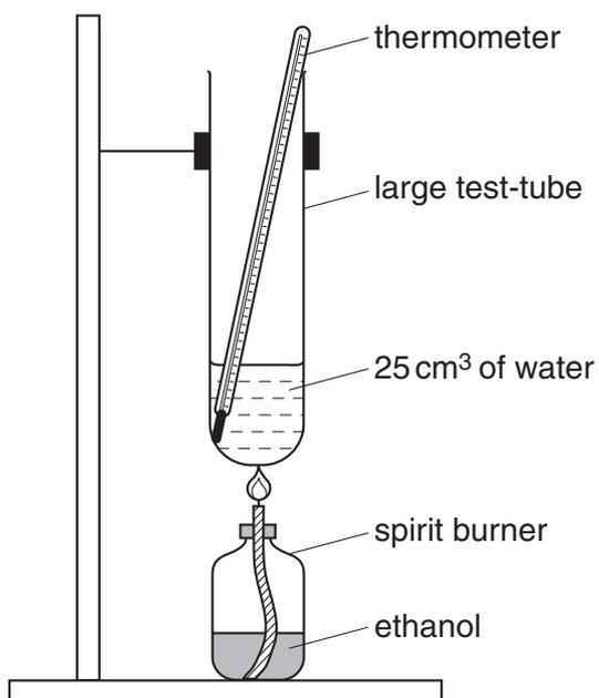
The mass of the burner and its contents is measured before and after the experiment. The thermometer is read before and after the experiment.
